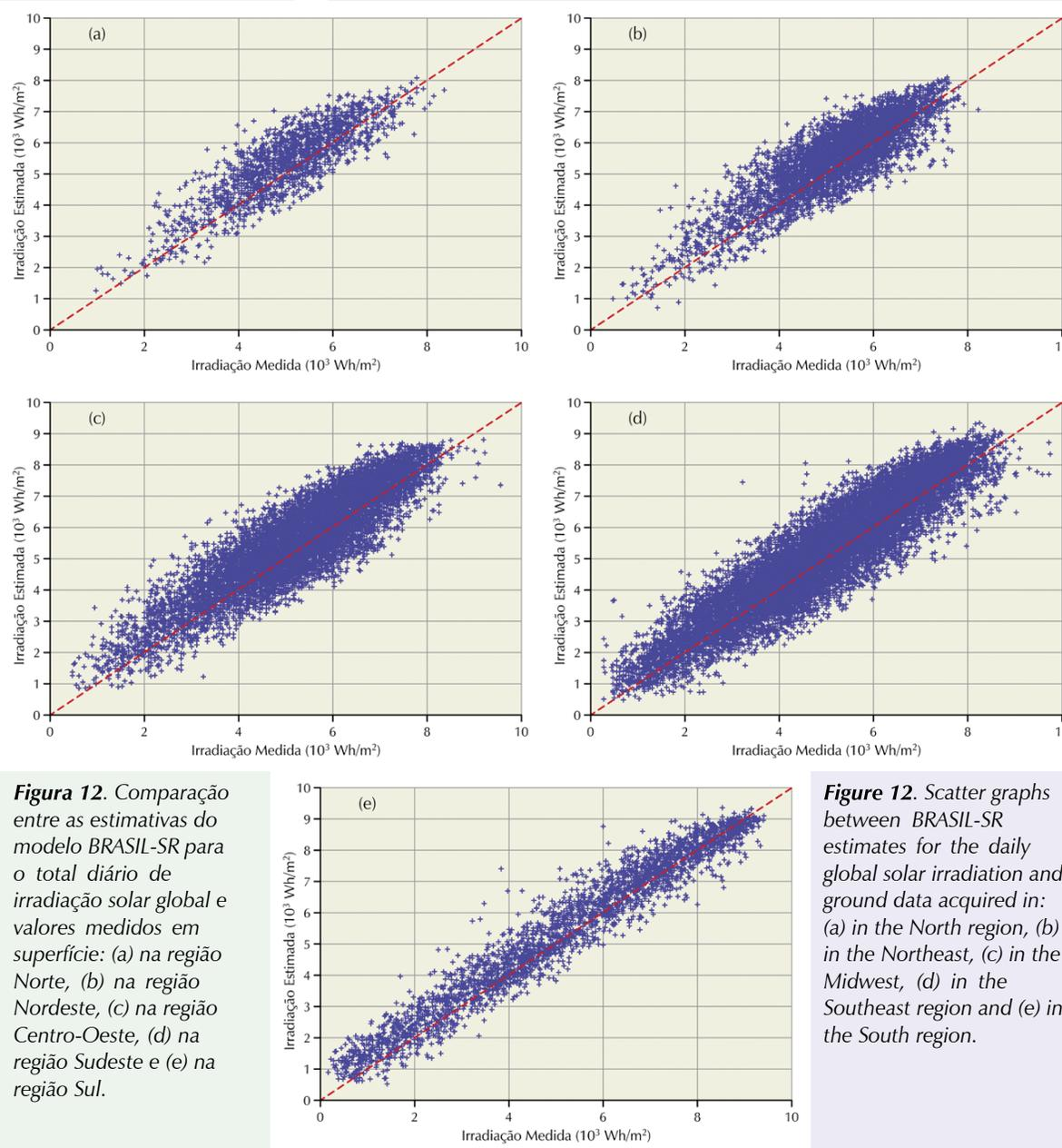
**Figure 12.** Scatter graphs between BRASIL-SR estimates for the daily global solar irradiation and ground data acquired in: (a) in the North region, (b) in the Northeast, (c) in the Midwest, (d) in the Southeast region and (e) in the South region.
