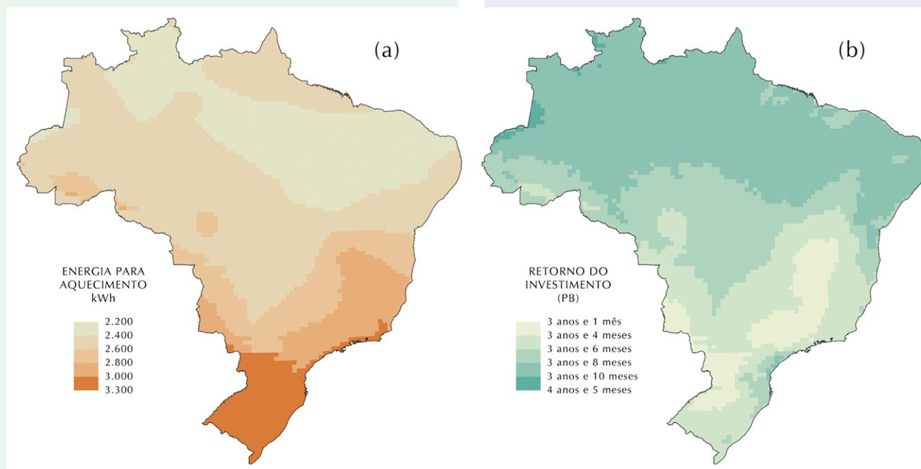
**Figure 19.** (a) Total required energy for water heating and (b) payback time (PB).
